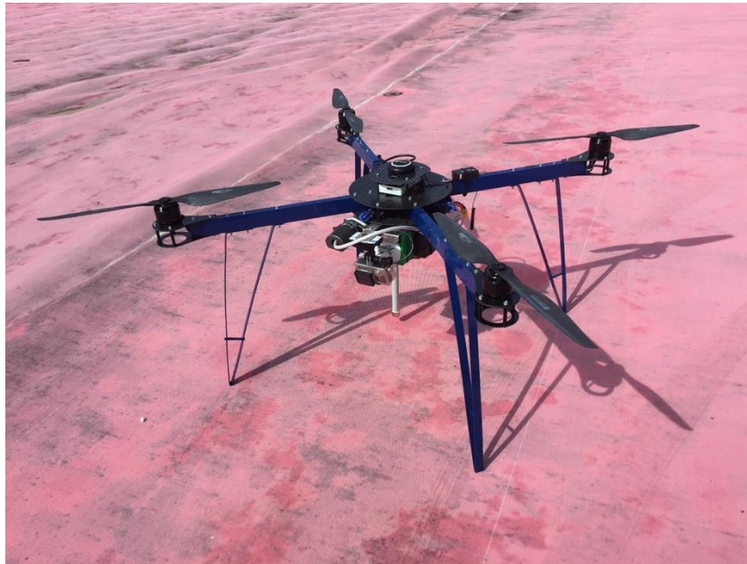
Figure 12: TEKEVER Multicopter VR3.5 with the installation of the antenna
