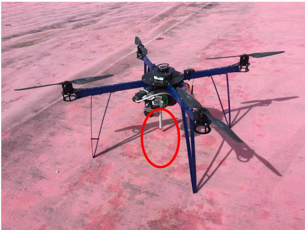
Figure 27: TEKEVER's VR3.5 multicopter with long range antenna
