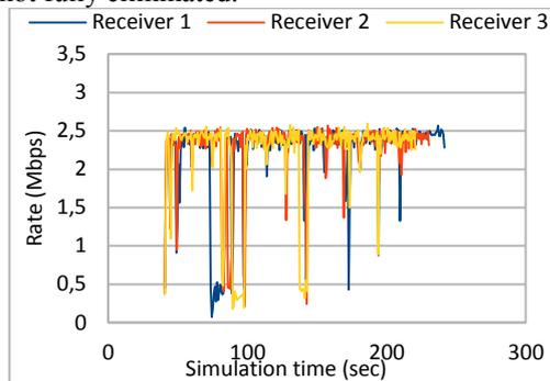
**Fig. 2.** Buffer Flush Output Rate for the Time-Based Mechanism with 3 Mobile Receivers and 40 KB TBO.
