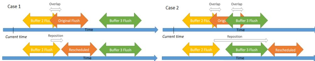
Fig. 2: Two cases of flush overlap avoidance using the Combined mechanism
