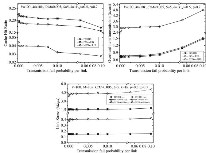
Fig. 10. The impact of the transmission link failure probability in the performance of the examined schemes.
