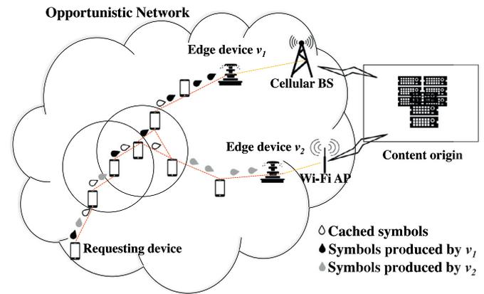
Fig. 2. Sending symbols from multiple devices through multiple paths.
